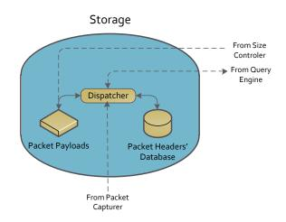
Figure 3. The Storage component. The dispatcher, in direct communication, with the Packet capturer gets raw packets and separates their payload and headers before storing them in two different blocks. It is also responsible of marshaling the GET requests of the query engine
