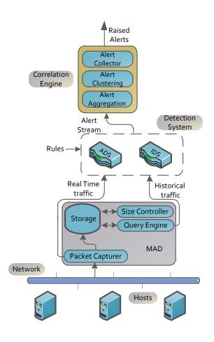
Figure 2. The MADs system overview. It consists of four main components: Packet capturer, Query engine, Size Controller and Storage. It aims to help traditional detection systems correlate the historical traffic with the real-time traffic in order to successfully detect sophisticated multi-step attacks.
