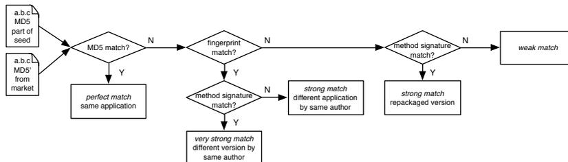
**Figure 6:** Flow chart of AndRadar’s application matching.
