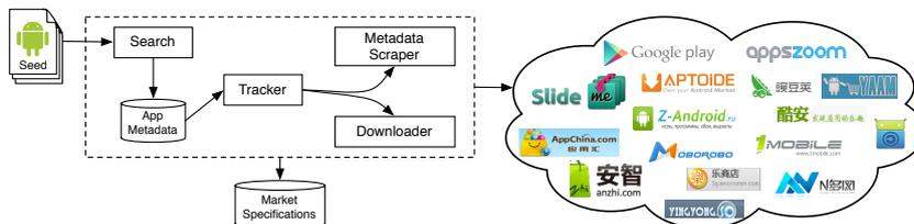
**Figure 5:** Overview of AndRadar’s architecture: The *seed*, which is composed of apps that have been flagged as malware, is used as input to the *search* for locating apps across markets. Once an app is found, the *tracker* downloads and stores additional metadata.
